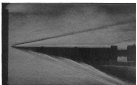
FIGURE 4. Schlieren photographs of model at various times during the nozzle starting process.
